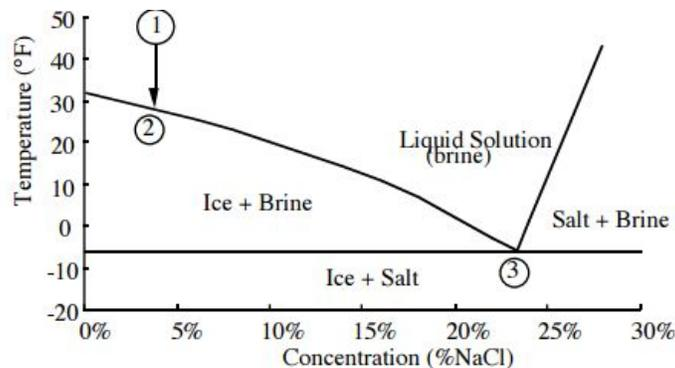
Figure 1. Phase diagram. Seawater at point 1 is first cooled to point 2, where water ice crystals begin to form. Further cooling results in increasing salt concentration until the eutectic at point 3 is reached.
