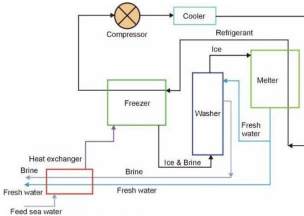
Figure 2. Sample Cryodesalination System
