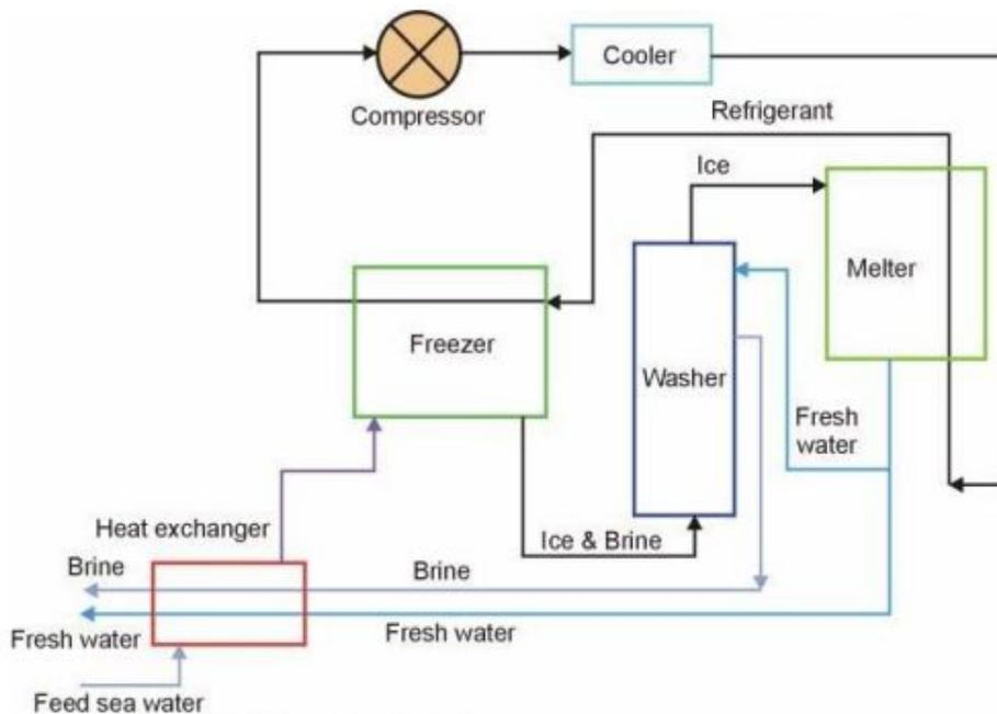
Figure 4: Sample Cryodesalination System
