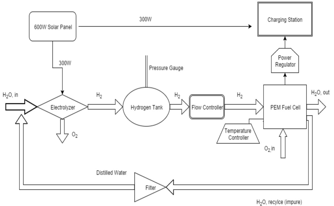
Figure 1: Design Diagram for 'Fuel Your Sol'
