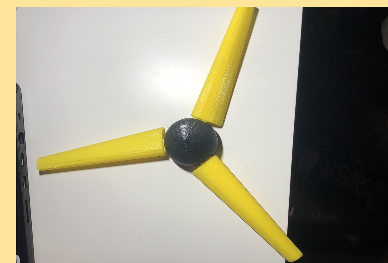
Figure 5: 3-D print of horizontal blades and hub.
