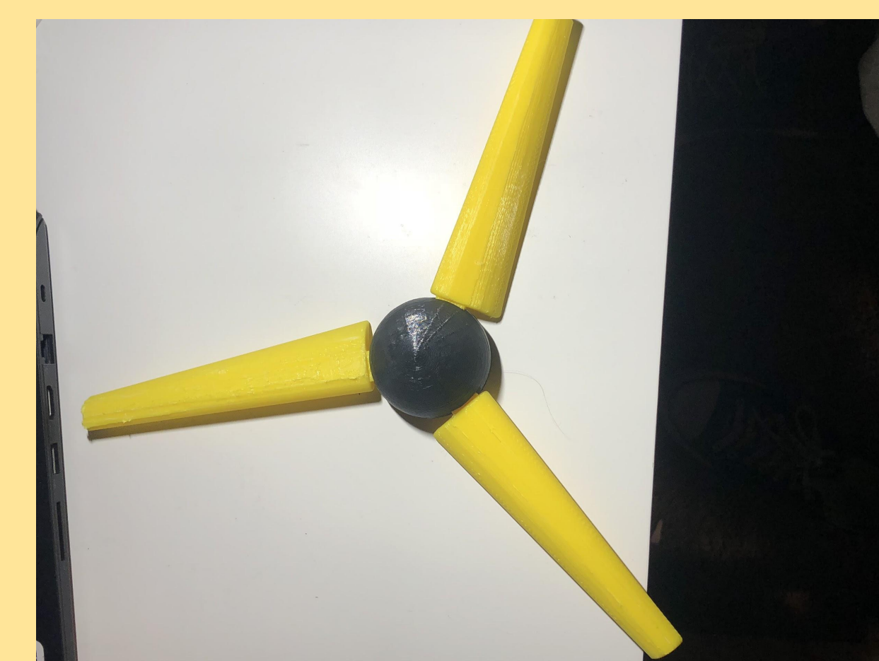
Figure 5: 3-D print of horizontal blades and hub.
