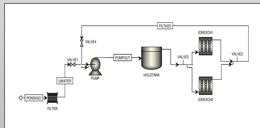
Our final system, diagrammed in the Aspen model above, will first flow the contaminated water through a filter to rid the water of relatively larger debris. The water will then flow through two exchange columns, which after several cycles, will store purified water in the holding tank.
