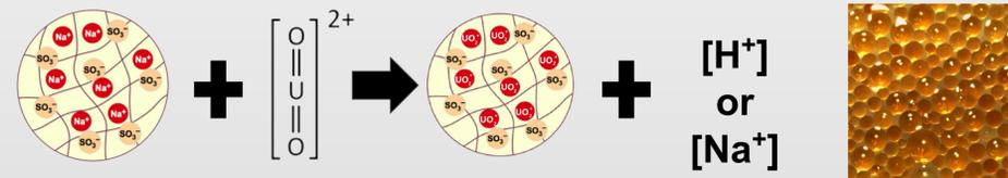
Contaminated water is pumped through a packed column filled with beads that adsorb uranyl and other contaminant ions.
