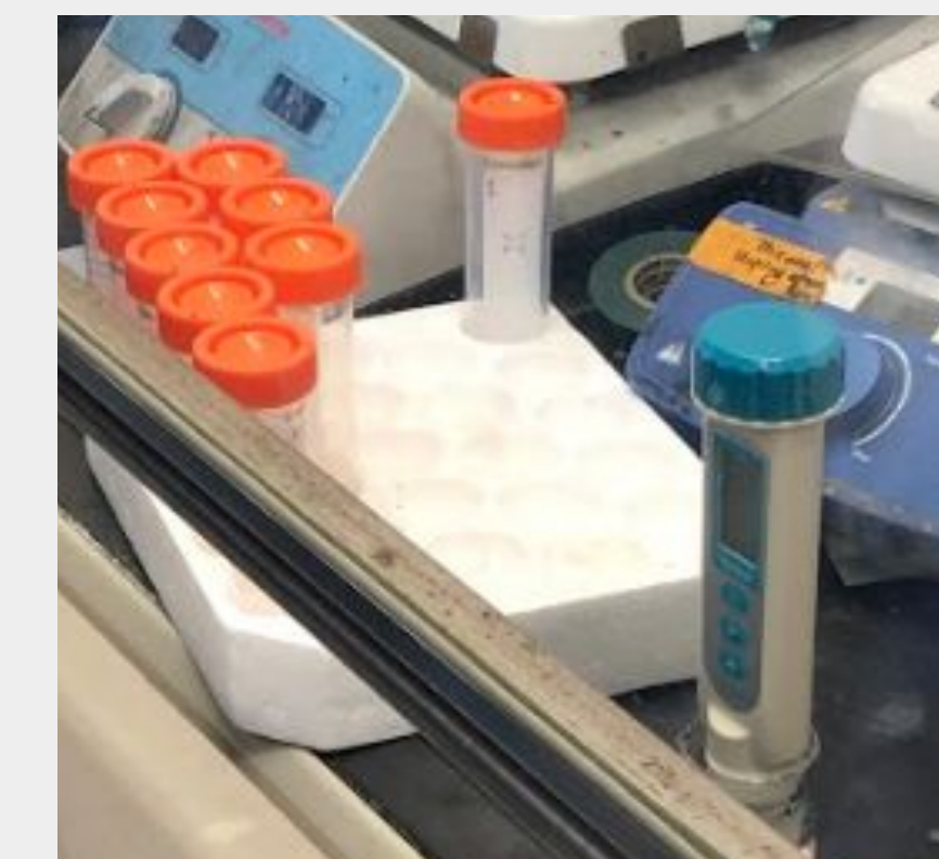
Fig. Taking conductivity measurements with known concentrations.
